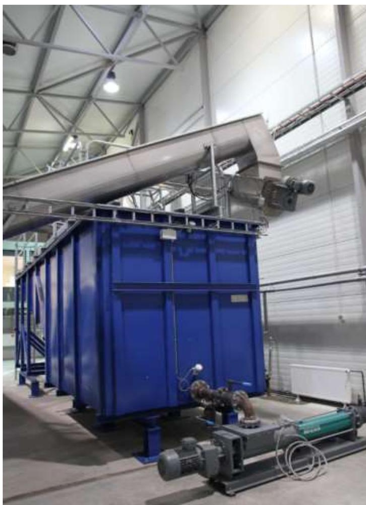
**Figure 4: Picture of the sink tank**
