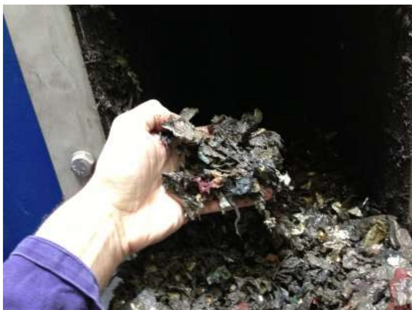
**Figure 3: Picture of plastic film after cyclone in hand**
