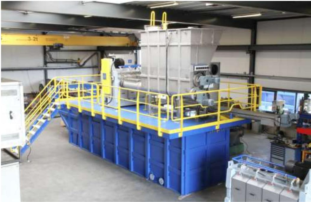
**Figure 5: Picture of the full cleaning system with the cyclone and sink tank**
